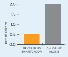
Silver plus 0.5 - 1.0 ppm of SmartChlor is as effective as 2.0 ppm of chlorine alone.
